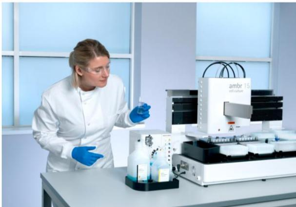
Caption: ambr® 15 cell culture system with ambr® analysis module showing BioPAT® Spectro port; to which a probe for Raman spectrometer is connected
